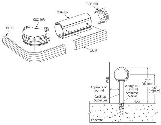
Drill 1" (25mm) dia. hole 3.25" (76mm) deep. Add anchoring cement per instructions insert sleeve until flush with floorWipe away exess cement.
